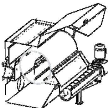
The key part of the system is a filtrating rotary drum with a mesh opening ranging from 0.25 to 4 mm.
